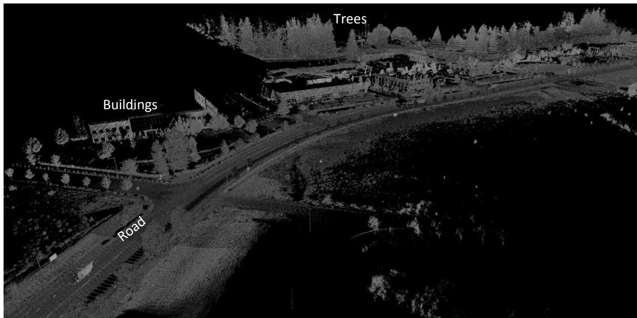
FIGURE 1 Example of a point cloud acquired by mobile LIDAR.
