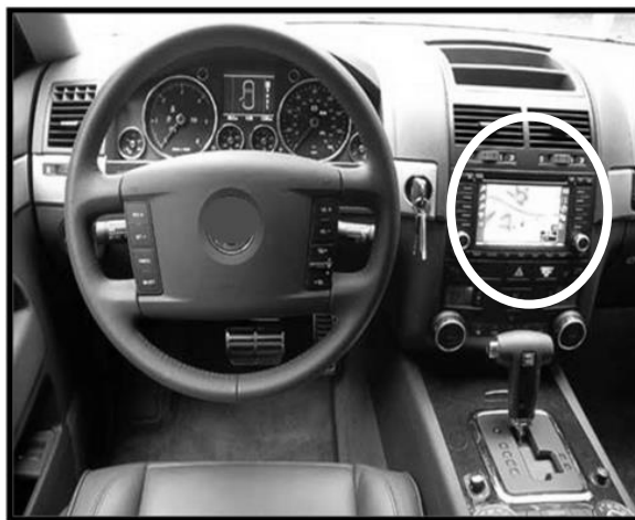
260 Figure 2 The interior of the test vehicle with rear camera view in the center console. 261
