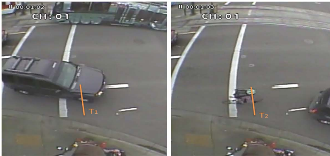
Figure 4.9: Post Encroachment Time (PET) = (T_2 - T_1) .
