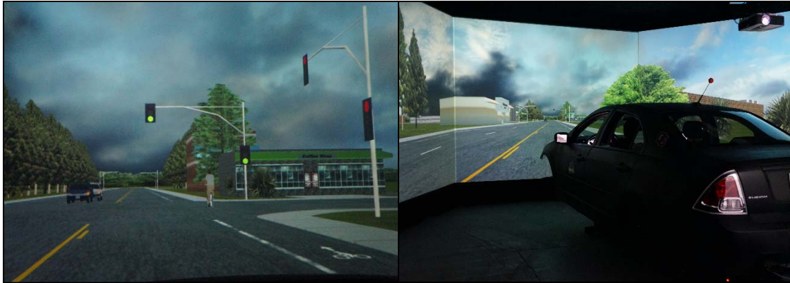
Figure 4.2: Simulated environment in OSU driving simulator.
