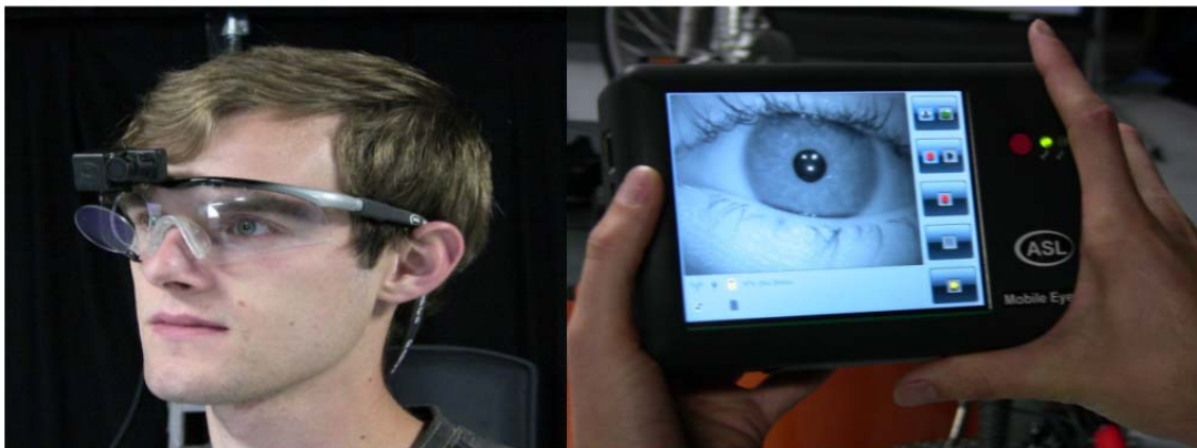
Figure 4.3: OSU researcher demonstrating the Mobile Eye XG Glasses (left) and Mobile Recording Unit (right).
