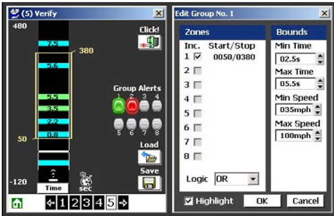
Figure 29 Manually established thresholds for Dilemma Zone
