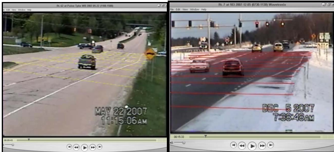
Figure 14 Digitized Video with Measurement Zones
