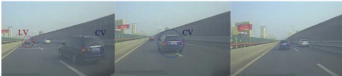
Fig. 3. Radar target T0 change, detecting a cut-in of the blue car from adjacent lane (For interpretation of the references to colour in this figure legend, the reader is referred to the web version of this article).
