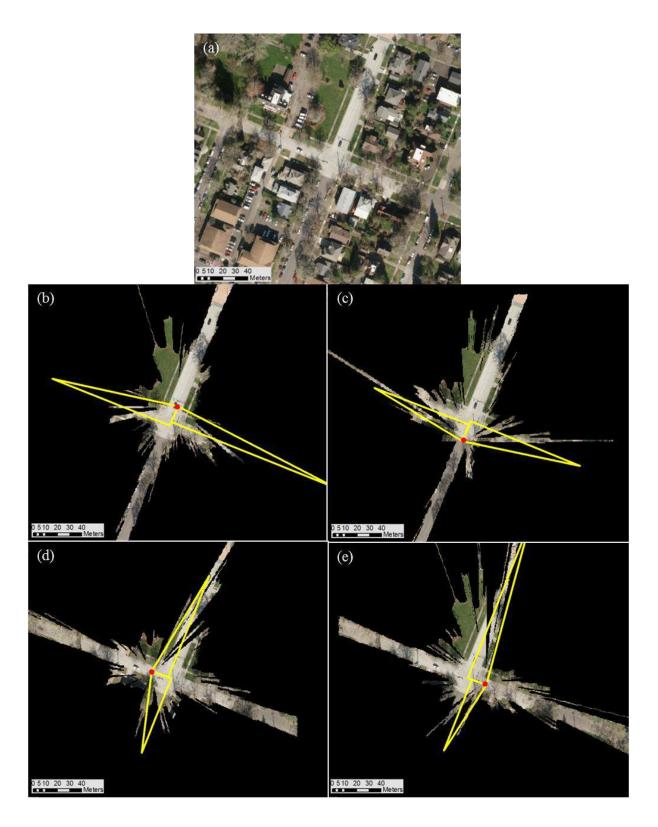
**Figure 5.3** Stopping sight distance triangles overlain on the visible scene determined with theSiDAL algorithm for the Jefferson intersection evaluating each traffic approach (a) North, (b) South, (c) West, (d) East.
