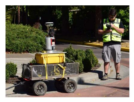
Figure 3.3 STLS mobile wagon set-up for stop-and-go scanning of the intersection.
