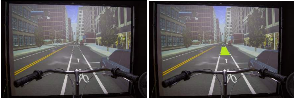
Figure 0.4 Two levels of pavement marking (adopted from NACTO, 2011). Left: White lane markings. Right: Solid green
