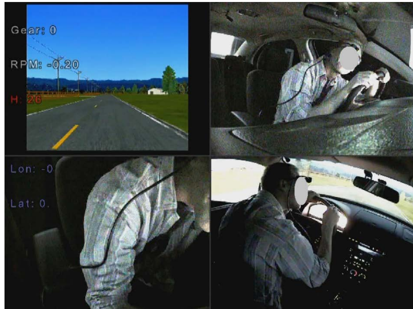
Figure 4.7: Example of participant leaning over the steering wheel to look at a drone operation. Top left: Simulated scene as projected on the screen. Top right: Driver leaning over the steering wheel. Bottom left: View of the driver’s torso leaning forward. Bottom right: Driver turning his head to the look at the drone operation.
