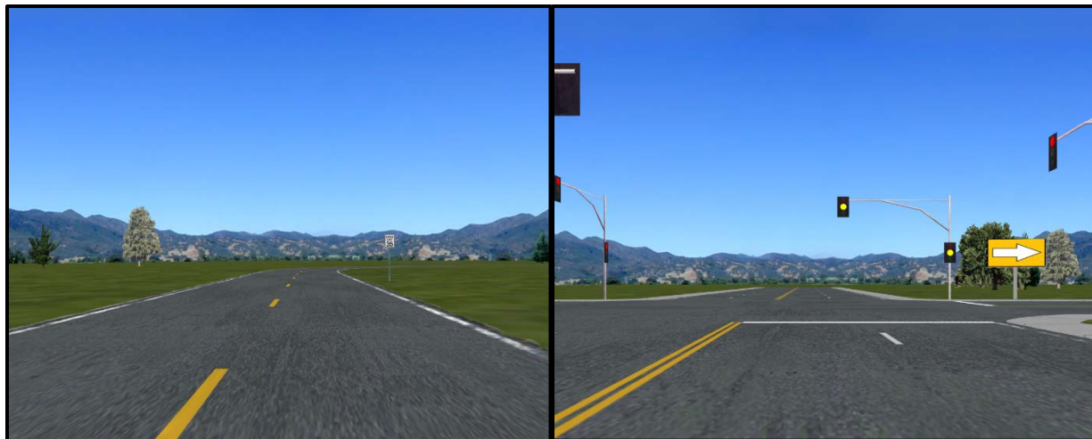
Figure 3.13: Screenshots of calibration drive in simulation. Left: Approach to a curve near the beginning of the drive. Right: Approach to a signalized intersection, where a yellow billboard indicates a right turn
