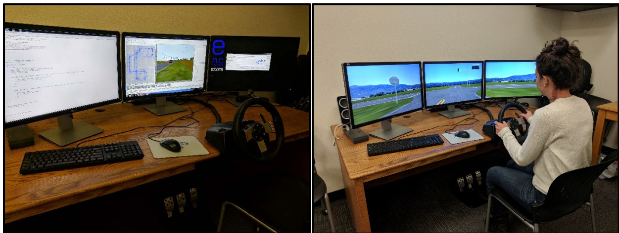
Figure 3.1: Operator workstation for the driving simulator. Left: Designing an experiment in the Internet Scene Assembler with Java script. Right: A researcher evaluating a newly designed environment.
