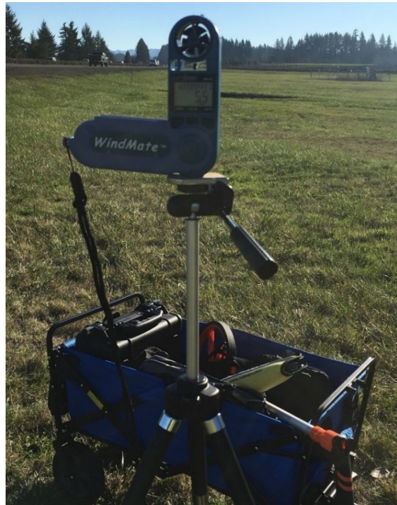
Figure 4.14: Instrument for measuring temperature, wind speed, and direction
