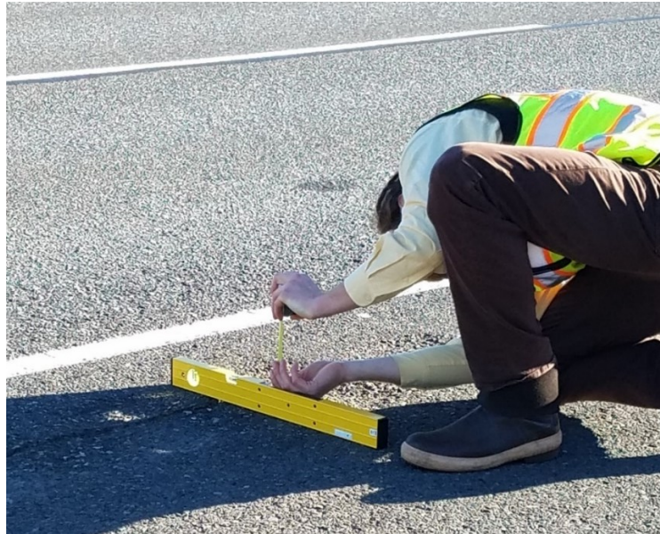
Figure 4.25: Measuring the depth of an individual mill
