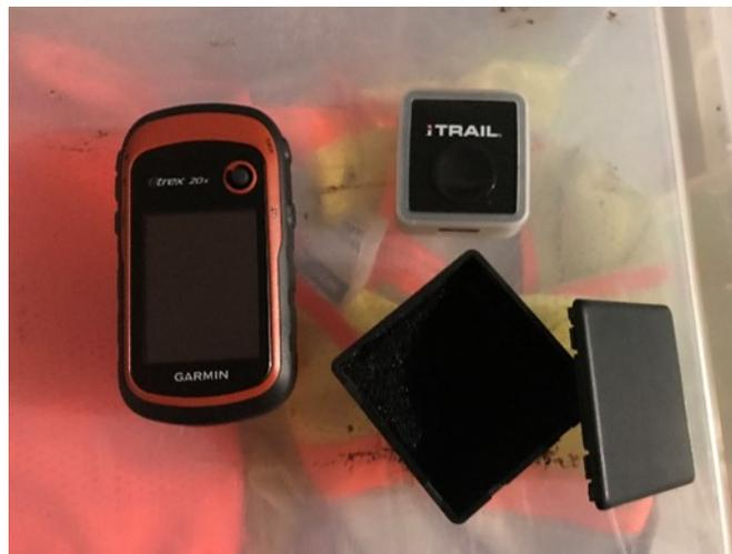
**Figure 3.6: Handheld GPS device (left), and GPS tracker and casing for GPS tracker (right)**
