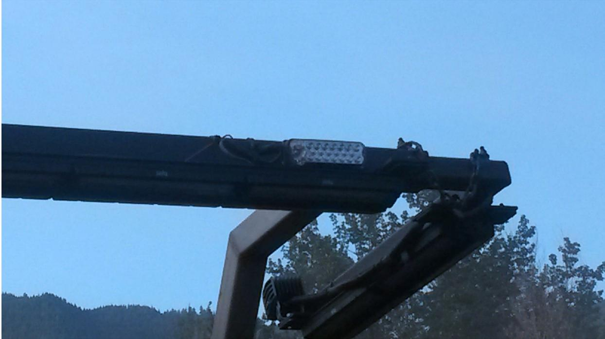
**Figure 4.2: Blue light installed on paving equipment**
