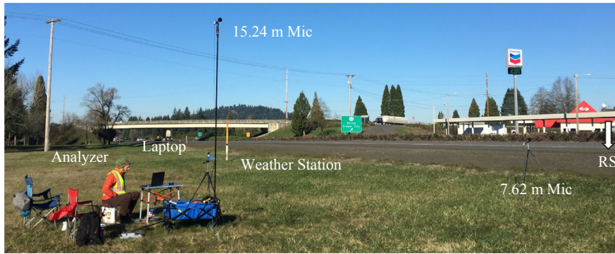
Fig. 3. Exterior sound measurement setup.
