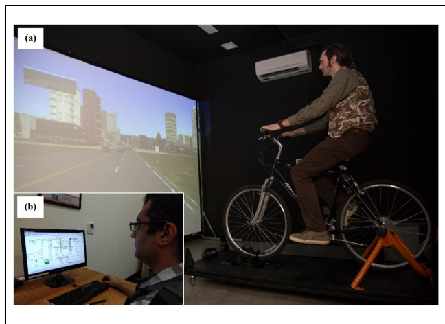
Figure 2. Views of the OSU bicycling simulator (a) and operator workstation (b).
