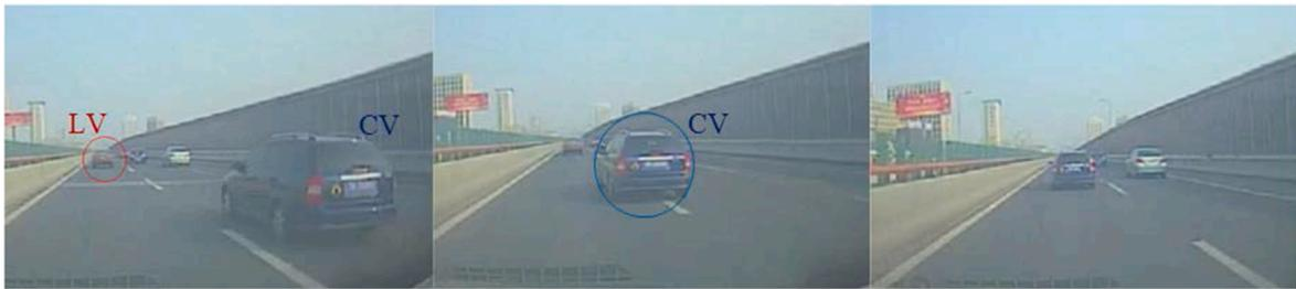
Fig. 2. FV radar target T0 change, detecting a cut-in of the blue car from adjacent lane.
