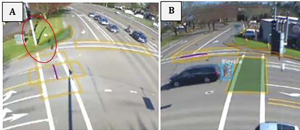
Fig. 5. False Detection Triggered by Signal Head Shadows (A) and a Bicycle Mounted on a Rear Bike Carrier (B) on the Optical Sensors.
