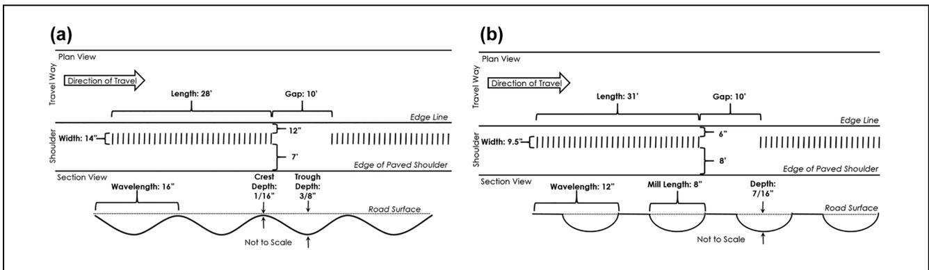
Figure 6. Typical geometric characteristics for (a) sinusoidal rumble strips (RS); (b) rounded RS
