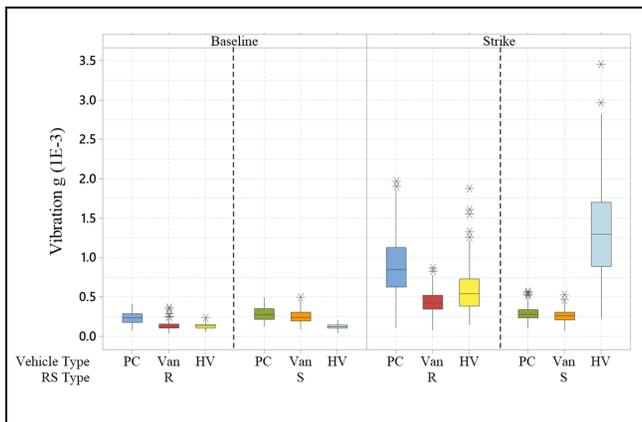
**Figure 15.** Boxplot comparison of vibration measurements.
