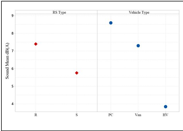
**Figure 10.** Main effect factors of interior sound measurement. Note: PC = passenger car; HV = heavy vehicle; RS = rumble strip.
