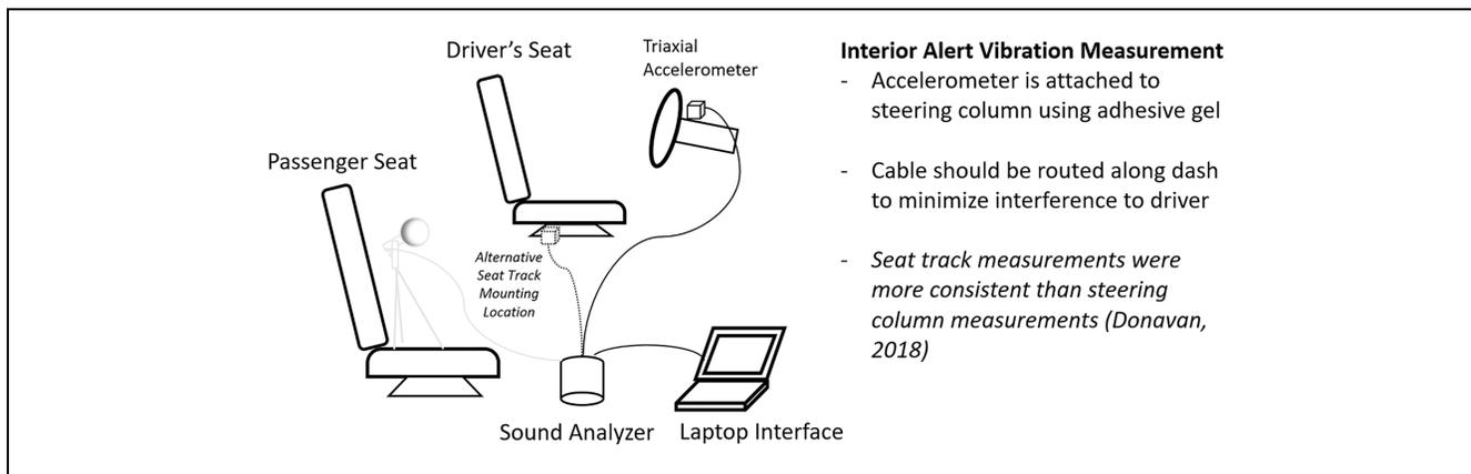
**Figure 2.** Interior alert vibration measurement diagram
