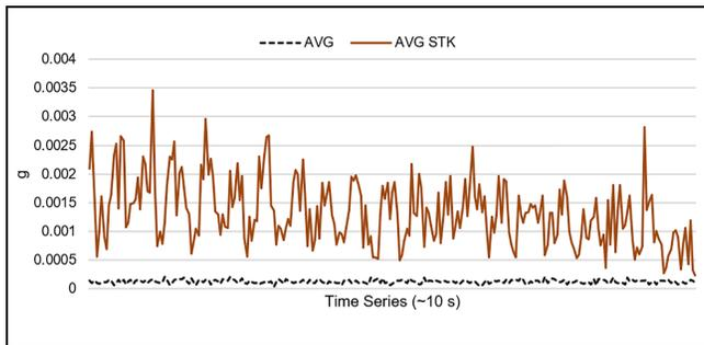
**Figure 14.** Vibration measurements for the heavy vehicle striking the sinusoidal rumble strip.
