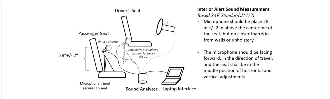
**Figure 3.** Interior alert sound measurement diagram.
