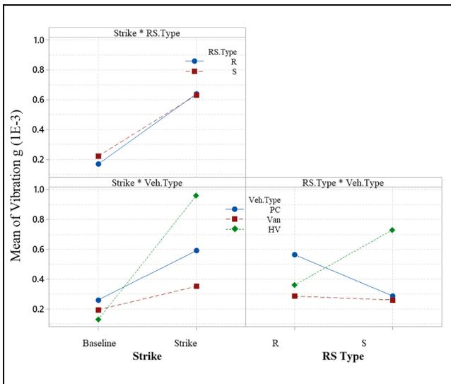
**Figure 17.** Two-way interaction plot of mean vibration by rumble strip (RS) type and vehicle. Note: PC = passenger car; HV = heavy vehicle.
