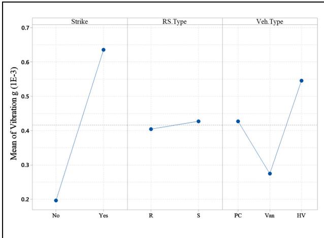
**Figure 16.** Main effect factors of interior vibration measurements. Note: PC = passenger car; HV = heavy vehicle; RS = rumble strip.
