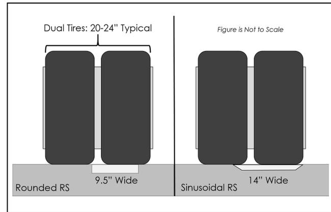
**Figure 18.** Bridging effect for dual-tire heavy vehicles.
