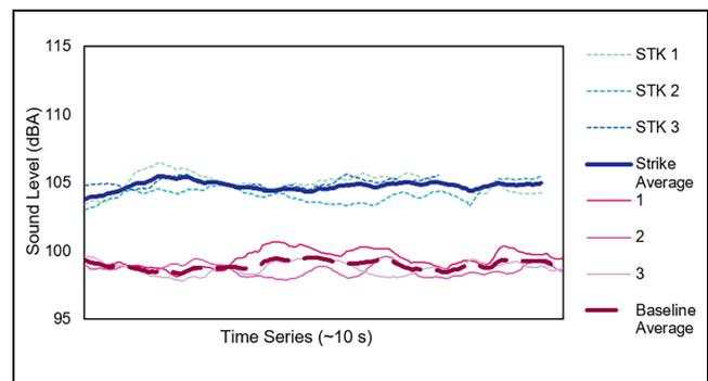
**Figure 8.** Interior sound comparison for the passenger car on the sinusoidal RS.
