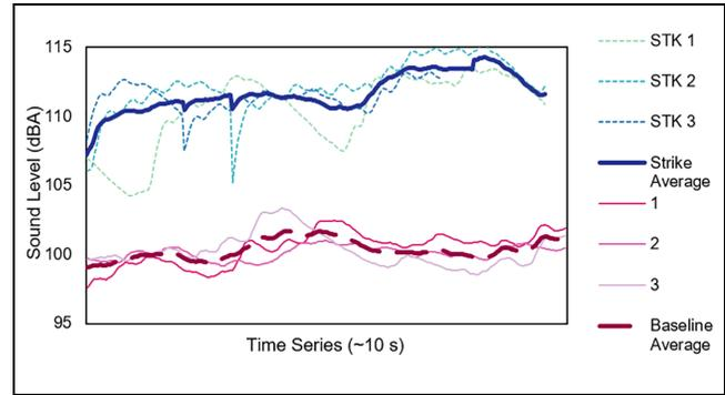
**Figure 7.** Interior sound comparison for the passenger car on the rounded RS.
