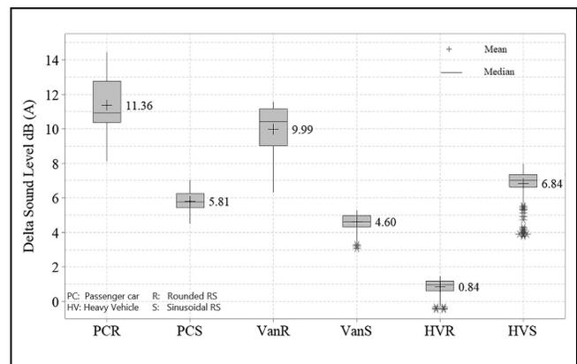
**Figure 9.** Boxplots by vehicle and RS type for interior delta sound measurements.
